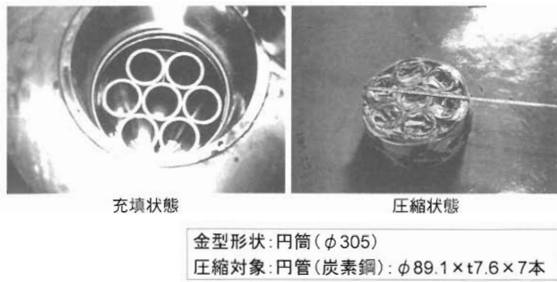
Fig.18 Result of 1000ton Compressing Test
